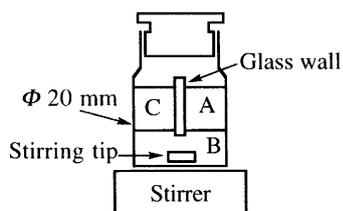
Fig. 3. U-Tube system for measurement of ion transport activity. The apparatus consists of a glass tube partly divided by a glass wall. The tube contained 1 ml of 7 mM calcium or sodium picrates (A), 3.5 ml of 0.5 mM test compound solution in water-saturated  $\text{CHCl}_3$  (B) and 1 ml of distilled water (C)
